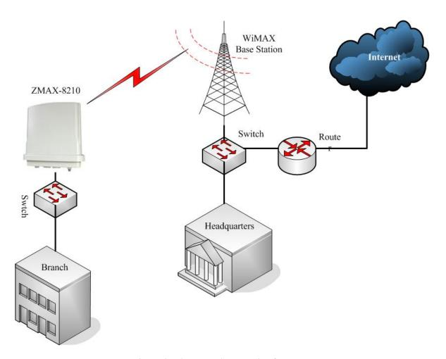
Figure 3 Wireless Point-to-Point Outdoors
